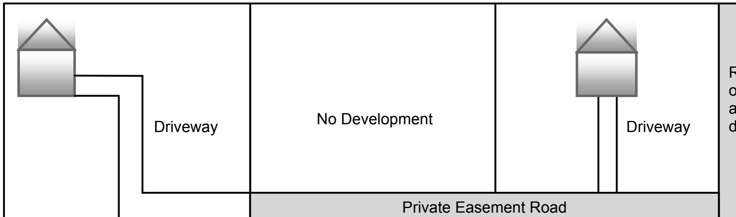
Figure 21-5 – Private Easement Road. In all zones, up to but not exceeding 3 properties may have their primary access by way of a “Private Easement Road”. Upon the fourth, it must become “Public Road” or “Private Road” depending on the zone and the primary use of the properties.
